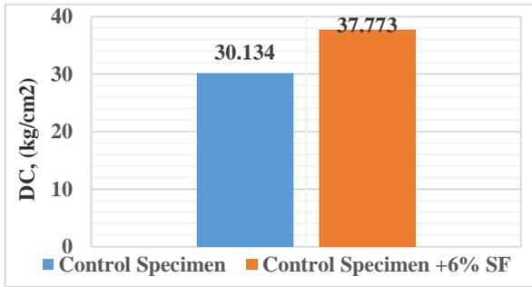
Figure (18): Effect of Adding SF on DC value
