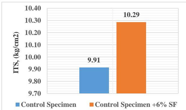
Figure (19): Effect of Adding SF on ITS Value
