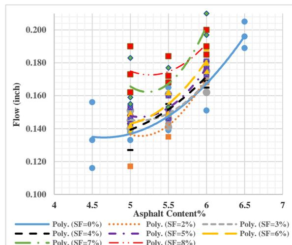
Figure (6): Effect of Adding SF on Marshall Flow Values
