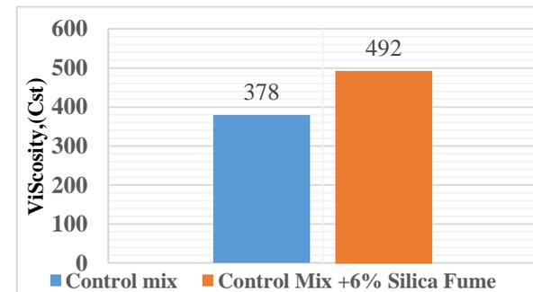
Figure (3): Effect of Adding SF on Bitumen Viscosity.
