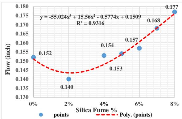
Figure (7): Effect of Adding SF on Flow Values (at OAC)
