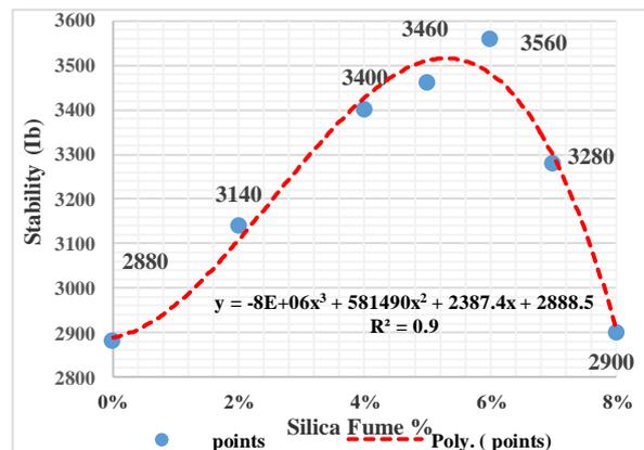
Figure (5): Effect of Adding SF on Marshall Stability at OAC
