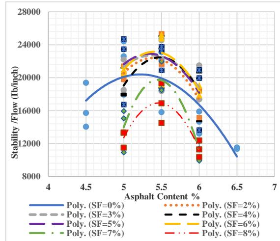
Figure (16): Effect of Adding SF on Marshall Stiffness
