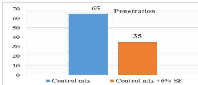
Figure (2): Effect of Adding SF on Penetration Value.
