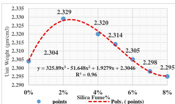
Figure (9): Effect of Adding SF on Marshall Unit Weight at (OAC)
