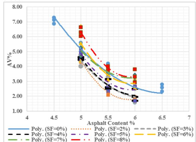
Figure (10): Effect of Adding SF on %AV
