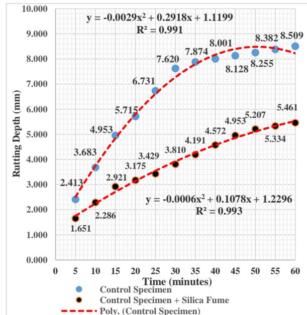
Figure (20): Effect of Adding SF on Rutting Depth
