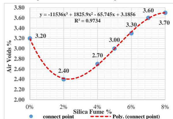
Figure (11): Effect of Adding SF on AV% at (OAC)
