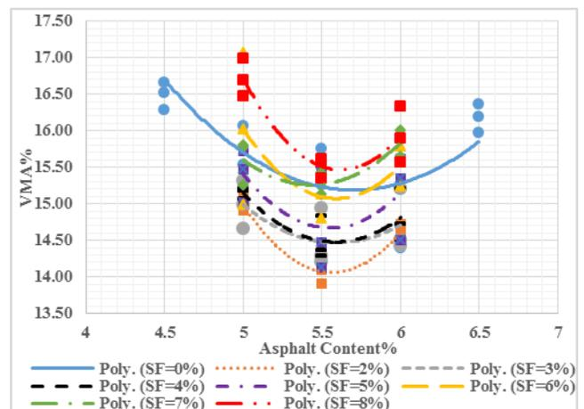
Figure (12): Effect of Adding SF on VMA%
