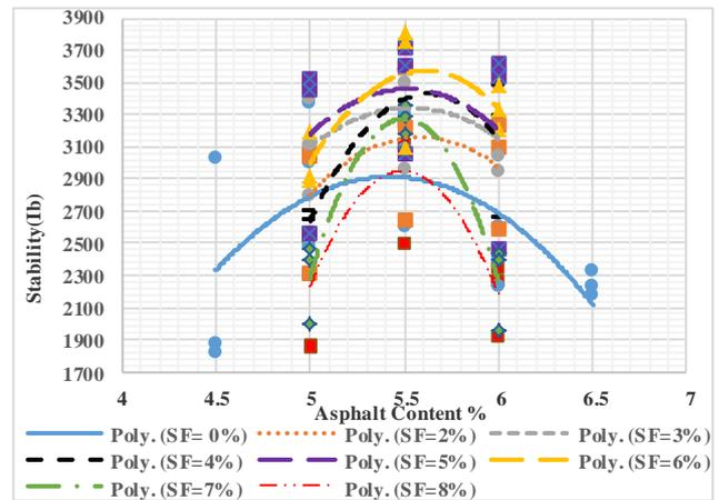
Figure (4): Effect of Adding SF on Marshall Stability
