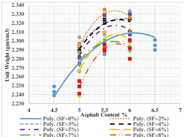
Figure (8): Effect of Adding SF on Marshall Unit Weight
