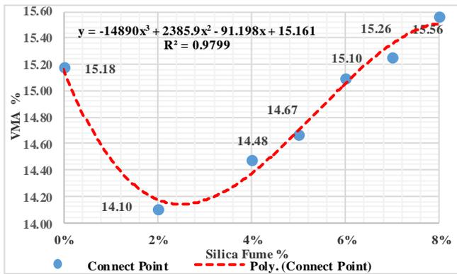
Figure (13): Effect of Adding SF on VMA% at OAC
