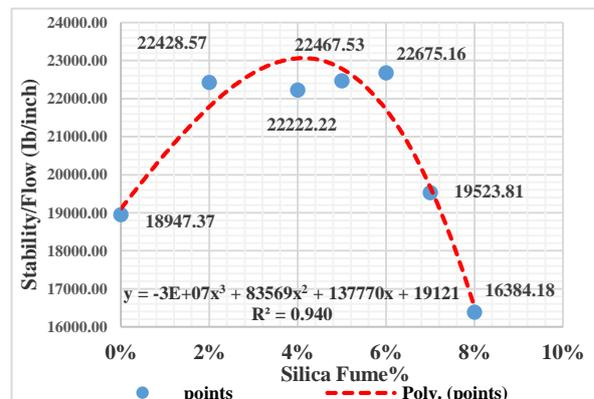
Figure (17): Effect of Adding SF on Marshall Stiffness
