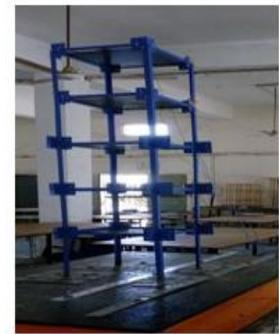
Fig 3 G+4 storey model without isolation
