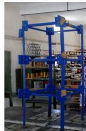
Fig 5 G+2 storey model without isolation
