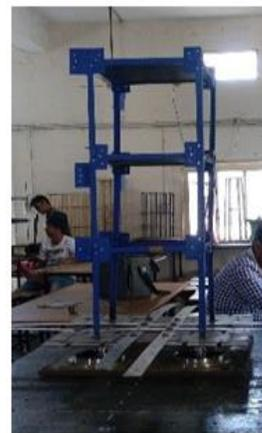
Fig 4 G+2 storey model with isolation
